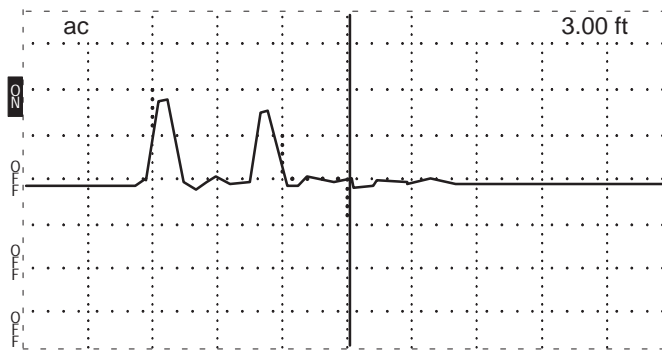
Figure 1-5: Vp Set at .30, Cursor Beyond Reflected Pulse (Setting Too Low)
